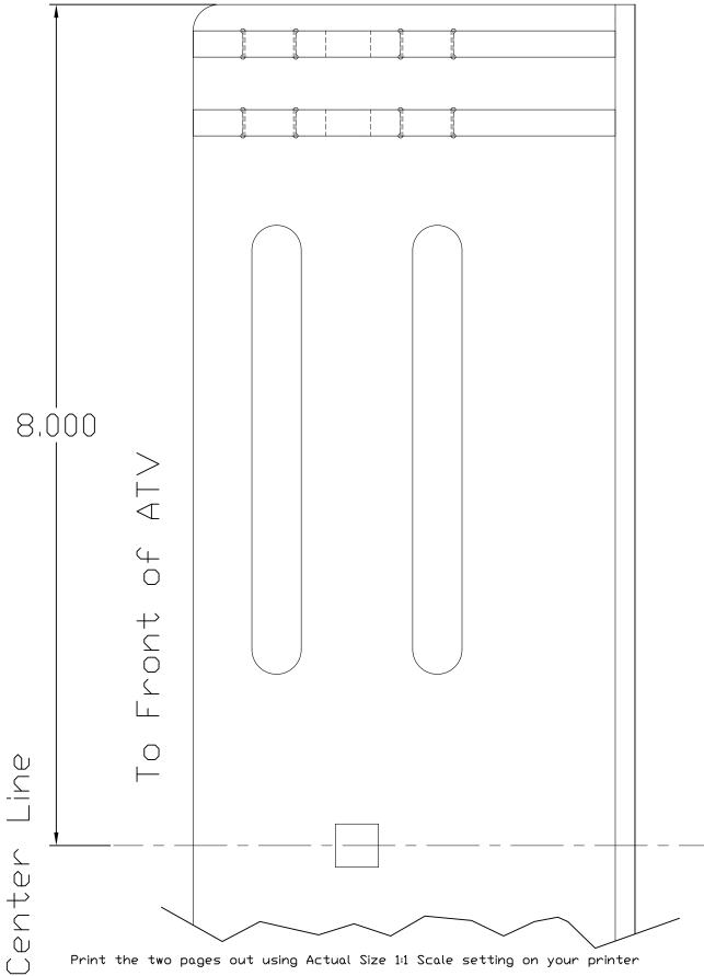
Verify the 8" measurment with a ruler to dertermine correct scale printed
