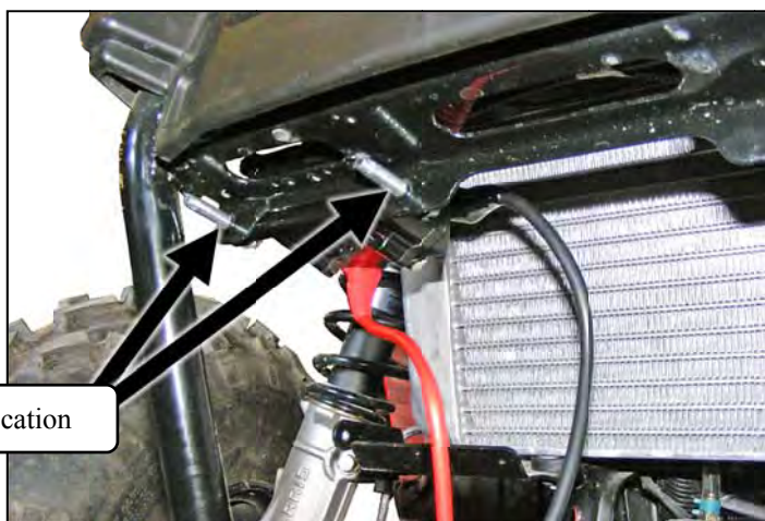
"Figure 8" 400/500/570/800 Contactor Location
