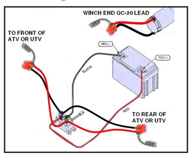
Optional Quick Connect Wiring Diagram
