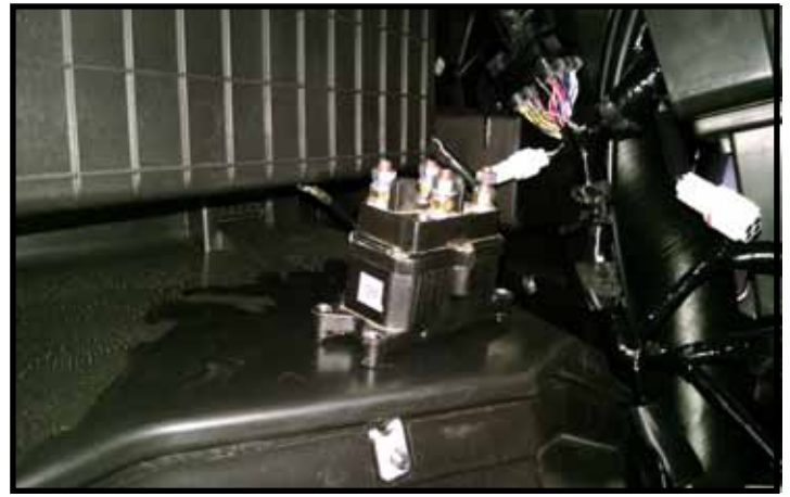
“Figure 11” Contactor Location Passenger Side Inner Wheel Well
