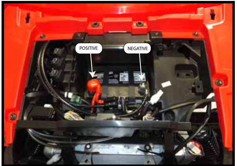
“Figure 9” Battery Location
