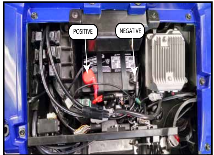
“Figure 12” Battery Location
