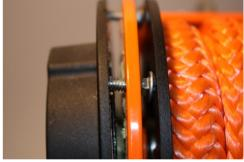
While one technician securely holds the spring housing, the second technician should insert a small flat screw driver or equivalent to pry the spring off of the shaft. NOTE: Make sure to keep the spring completely within the spring housing at all times. Failure to do so could result in serious bodily harm and/or damage to the surrounding room and contents.
