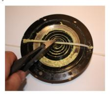
Identify shaft slot and spring flat. Align spring flat with shaft slot. Once spring flat is aligned with shaft slot, slide housing as far as possible towards base plate without engaging the screws.
