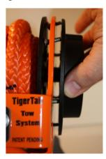
Rotate (less than a full turn) spring housing counter-clockwise until the text on spring housing is right side up and horizontal (parallel to base). Starting location may be different than illustrated. Rotate housing 3 additional counter clockwise turns.
