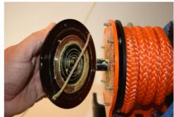
Thoroughly clean base plate surface and inspect for seal damage. If seal is damaged, refer to SECTION II of the manual for the seal replacement procedure. Inspect and clean spring/spring housing. If spring is damaged or can't be fully cleaned—purchase new spring and spring housing (p/n 41027-00). Clean and inspect o-ring for damage, replace if necessary (p/n 41024-00). Clean o-ring groove in spring housing.
