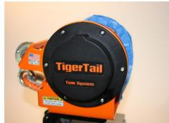
One technician should firmly grip the housing with both hands. To assist in a clean release of spring tension, the second technician should push all six machine screws toward spool to minimize the distance that the housing has to be from baseplate. Gradually pull housing off of fasteners (maintaining a firm grip) and allow the tension (3-4 rotations) in the spring to unwind slowly.
