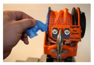
Remove TigerTail from secured work area and reinstall on vehicle. If the TigerTail was removed from the mount, the fasteners that are used to secure the TigerTail to the mount should be tightened to 78 ft-lbs of torque (clean, dry threads).
