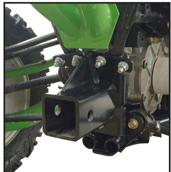
"Figure 3" Receiver Installed
