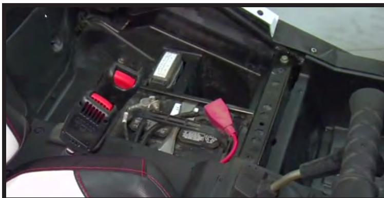
“Figure 13” Battery Location (Battery is located under driver seat.)
