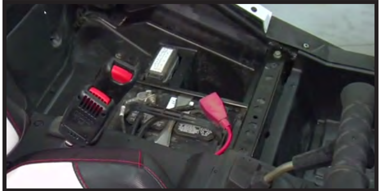
“Figure 14” Battery Location (Battery is located under driver seat.)
