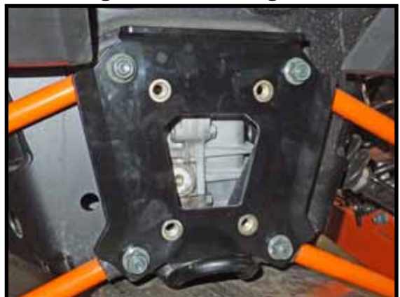
"Figure 4" Plate Install
