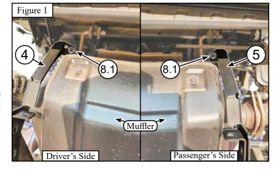
2. Place Upper Drivers Side Mount (4) in place as shown in **Figure 1**. Use Bolt (8.1) and Nut (8.2) to secure it. Repeat on the Passenger's Side Mount (5) as shown in **Figure 1**. Nut (8.2) is not shown in this image.
