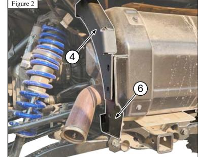
Note: Where the upper and lower bracket meet, the Upper Brackets should be on the outside of the Lower Brackets as shown in Figure 2.
