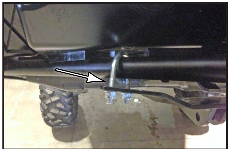
"Figure 5" Spacer Install
