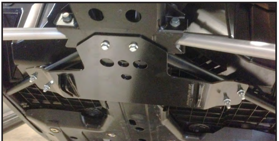
"Figure 6" Mount Plate Install
