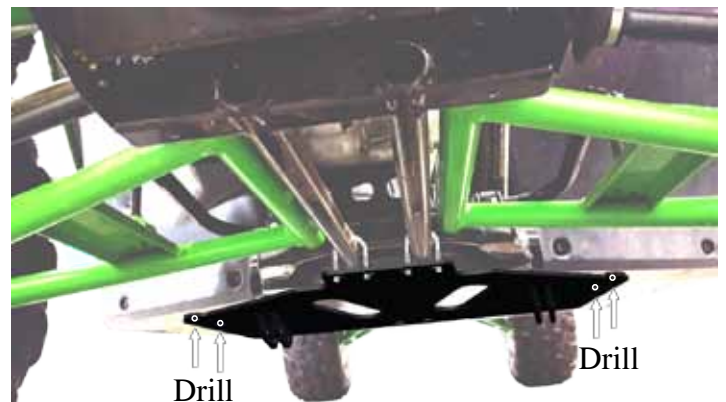
“Figure 3” Mount location/ where to mark for rear U-Bolts
