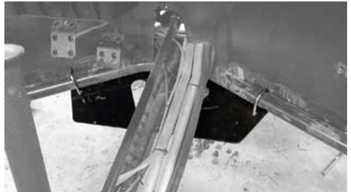
“Figure 5” Rear U-Bolt locations (Inner-floor & Skid plate removed to show U-Bolts & mount location)
