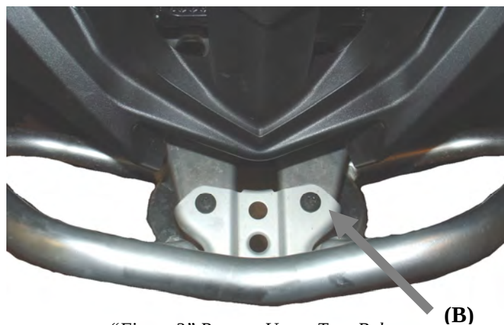
"Figure 3" Remove Upper Torx Bolts
