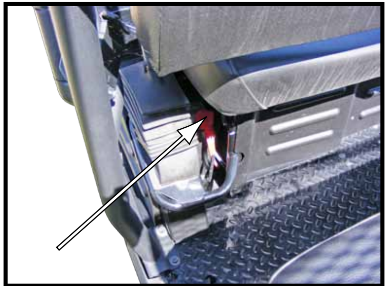
“Figure 9” Battery Location (Battery is located under driver side of the seat.)
