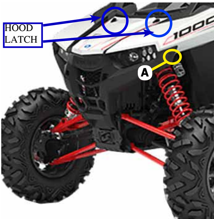
"Figure 2" Hood Removal
