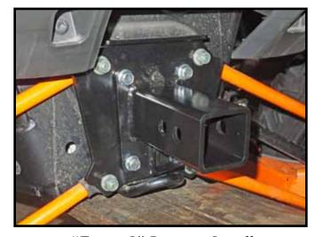
"Figure 5" Receiver Install
