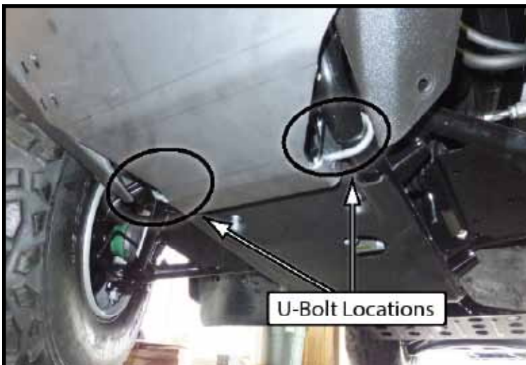
"Figure 3" U-Bolt Install
