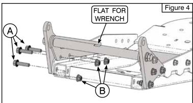
**Note:** When tightening bolts (5.5), use a 7/8" wrench or an adjustable wrench on the flat spot of rod (4) to prevent it from rotating. See **Figures 2 and 4.**
